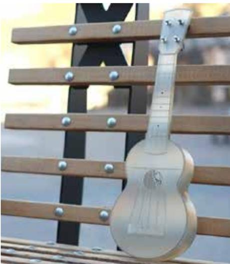
Realize Inc.'s project lead, Brian Cazzell, says that Outdoor Ukulele was having trouble finding someone who could build a full-scale prototype of its tenor ukulele using polycarbonate-like resin. The final instruments are injection-molded from glass-filled polycarbonate, and the prototype needed to be as close as possible in size and strength to the final instrument.
