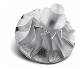
**5-AXIS MULTIBLADE LEVEL 2** provides incremental capabilities to 5-Axis MultiBlade Level 1 to machine parts that have multiple splitters and/or sub-splitters. It adds a fillet machining strategy and provides additional control for all toolpath strategies. (Requires 5-Axis MultiBlade Level 1)
