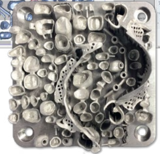
Dental tray designed using 3DXpert and printed in titanium
