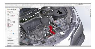
Verify design intent and accuracy. Check the accuracy of the model compared to the 3D point cloud.
