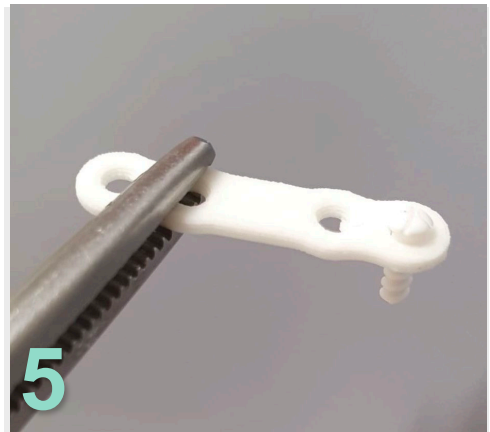
3D Printing of patient-specific osteosynthesis plates (Poly(L-lactide-co-D,L-lactide))
